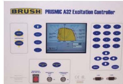
Automated Voltage Controller
